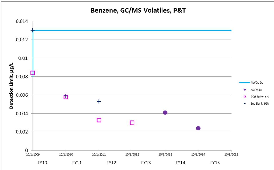
Figure 7. Plot of the detection limits (DLs) calculated by the various DL procedures for benzene, GC/MS volatiles, P&T.
