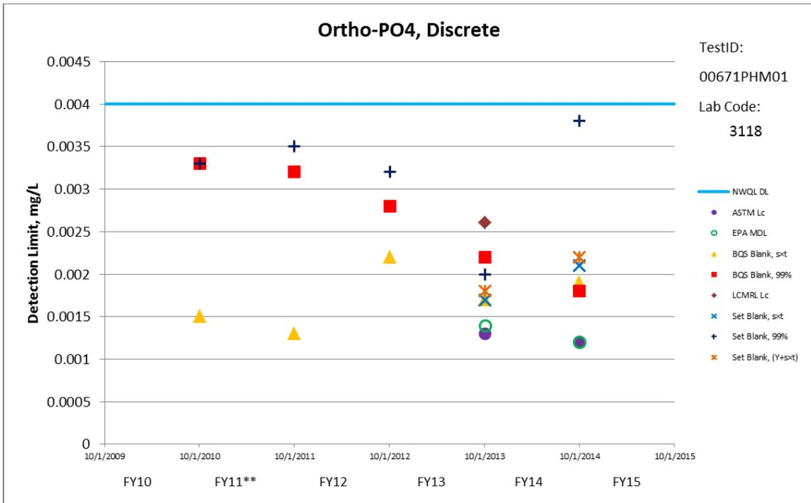
Figure 6. Plot of the detection limits (DLs) calculated by the various DL procedures for ortho-PO4, discrete.
