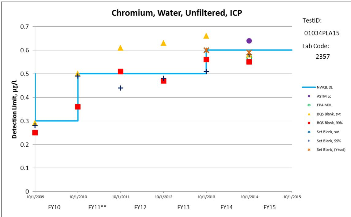
**Figure 2.** Plot of the detection limits (DLs) calculated by the various DL procedures for unfiltered chromium by ICP.
