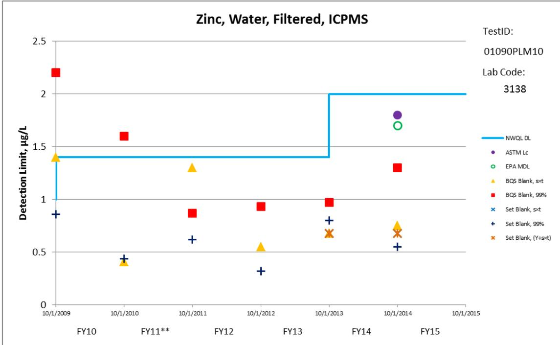
**Figure 3.** Plot of the detection limits (DLs) calculated by the various DL procedures for zinc, water, filtered, ICPMS.
