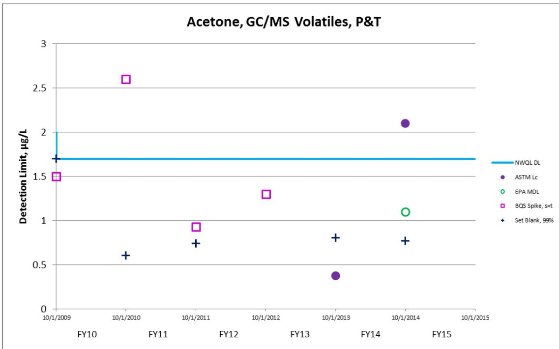
**Figure 8.** Plot of the detection limits (DLs) calculated by the various DL procedures for acetone, GC/MS volatiles, P&T.
