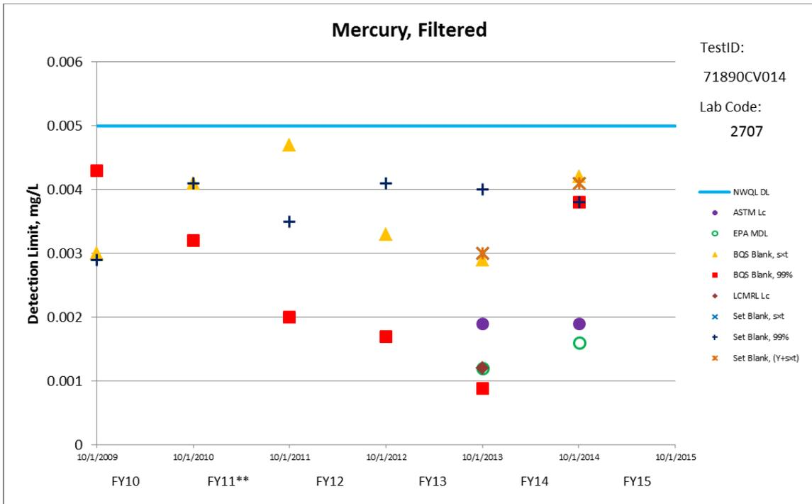
Figure 4. Plot of the detection limits (DLs) calculated by the various DL procedures for filtered mercury.
