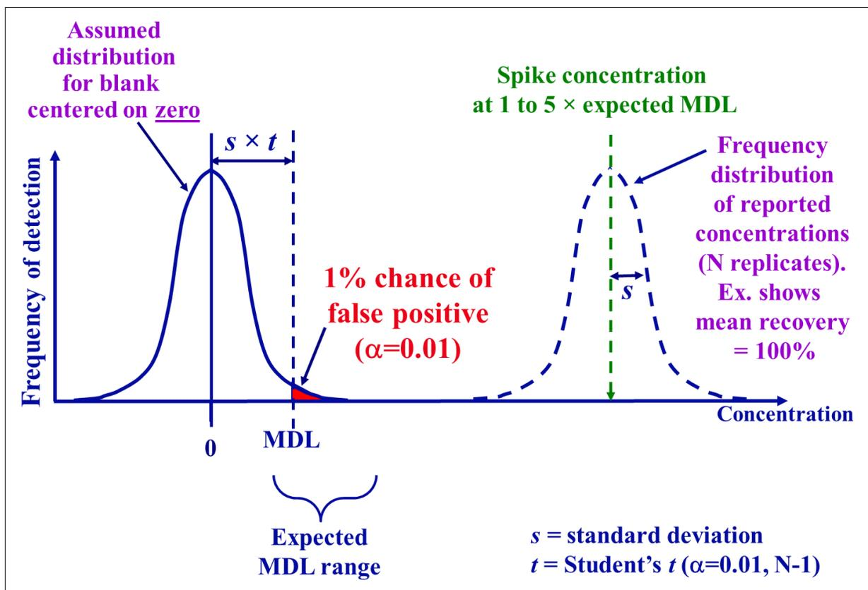
**Figure 1.** Determination of the method detection limit (MDL) or long-term method detection limit (LT-MDL) using spiked replicate samples.
