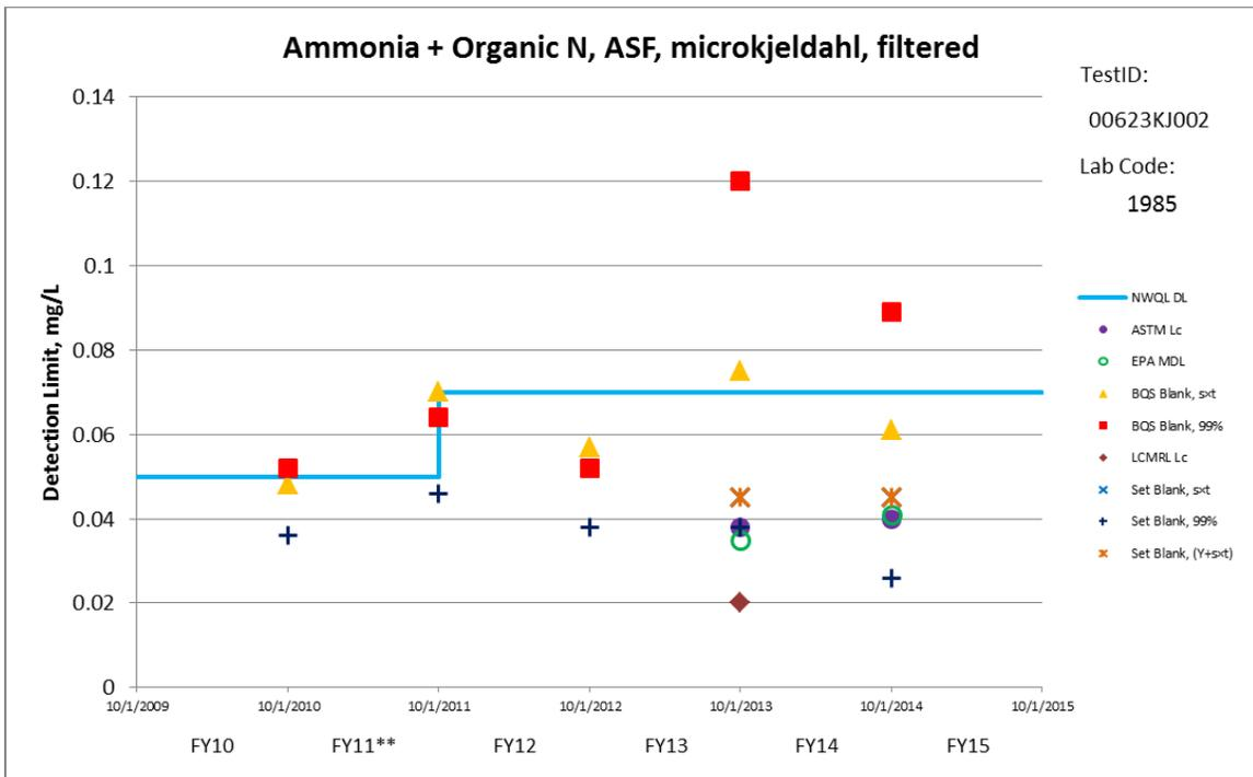
Figure 5. Plot of the detection limits (DLs) calculated by the various DL procedures for ammonia + organic N, ASF, microkjeldahl, filtered.
